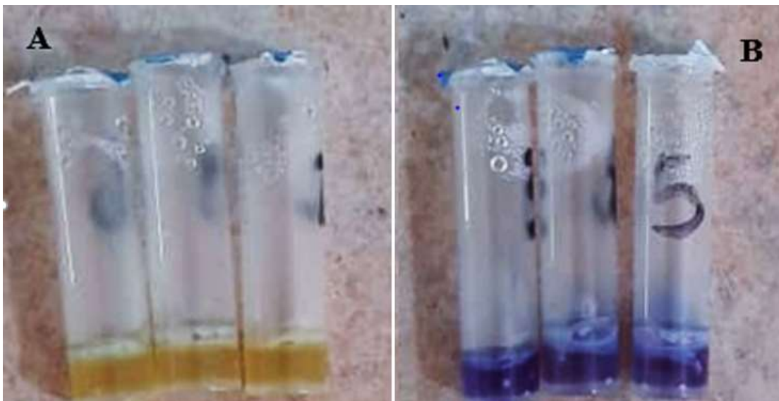
Figure 1: A) negative, B) positive Result: a purple color indicates the presence of antibiotics at or above the detection limits of the test
